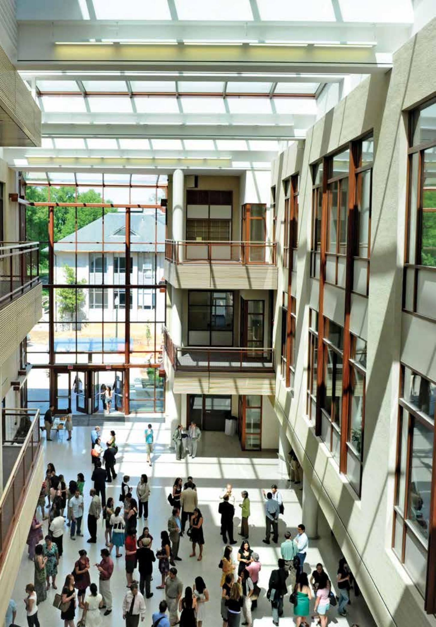
Natural daylighting through skylights and window walls is a key component to sustainability on campus. Photo courtesy American University.
